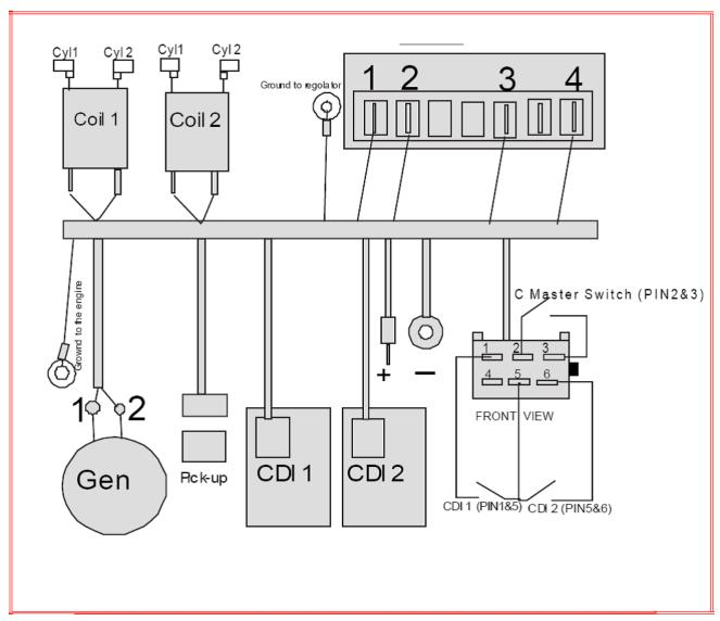
The white connector must be connected as shown in the drawing:
