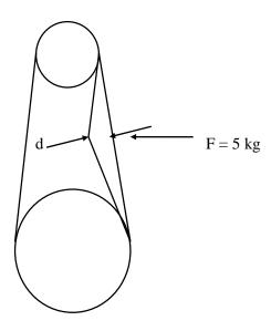
The belt should not move by more than 2 mm if a pressure of 5 kg is applied.
